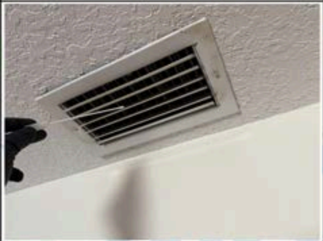
Interior Kitchen HVAC Vent Swab Sample
